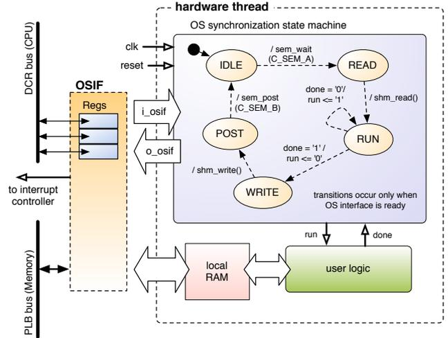
Fig. 1. Communication between HW thread and OSIF
